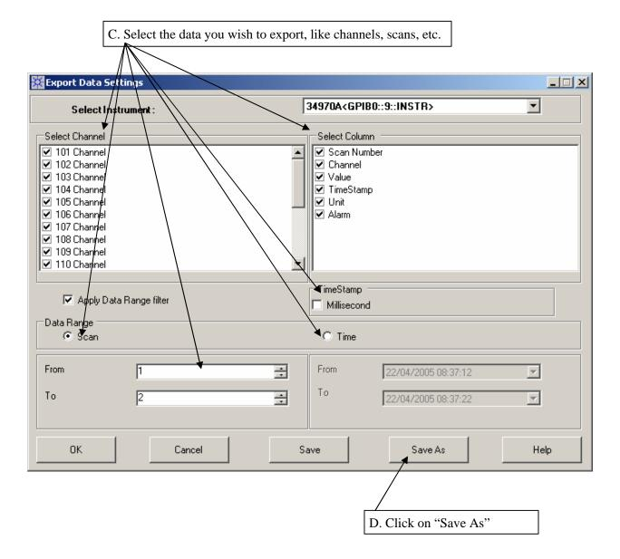
6. The data can now be saved in a different data format. Select either the .CSV or .TXT file format. Either format can be loaded into Excel.
