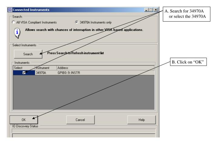
3. Configure instrument using the instrument upload configuration, as follows
