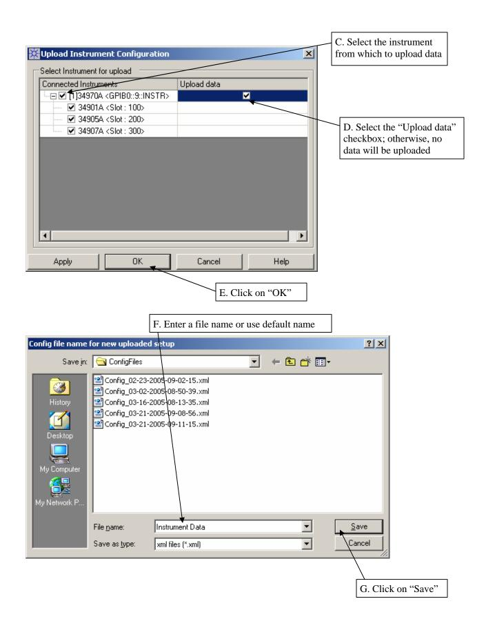
4. The instrument setup and data is next uploaded. When completed, the program displays the following window:
